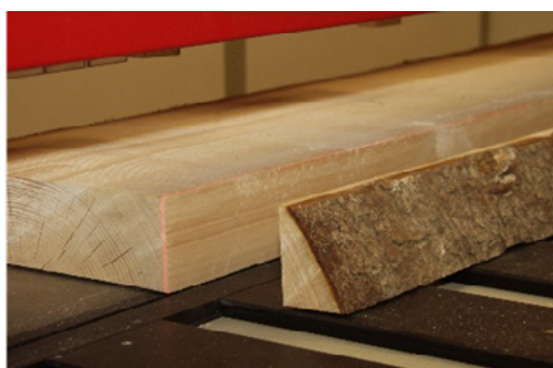
2/ Longitudinal cuts (trimming)
