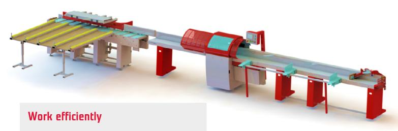
Solution for single worker operation. The operator prepares the material for the transverse extension. It inserts the material into the cut, during the material cutting process it has enough time to prepare more material at the inlet. The output roller conveyor picks up the material behind the cut and with the help of the puncher the material is moved to the gravity chute or to the box.
